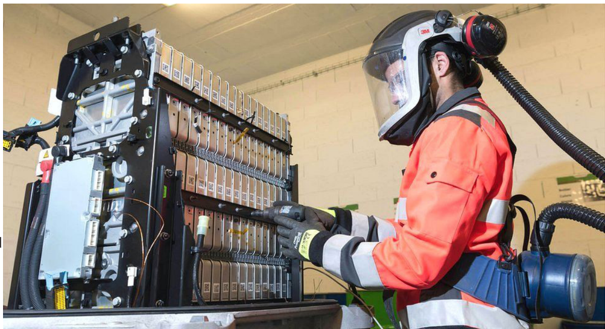
Serious PPE for a technician dismantling an EV battery at Renault’s facility.
